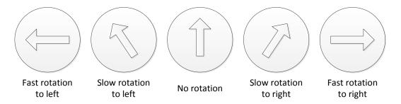
In addition to using the potentiometer to control direction and speed of rotation, this exercise should use the switch to enable and disable rotation. If the switch is pressed while the LEDs are rotating, the system should pause in its current position, regardless of whether the ADC input value changes. If the switch is pressed while everything is paused, the system should resume rotating in the appropriate direction based on the ADC input value.
