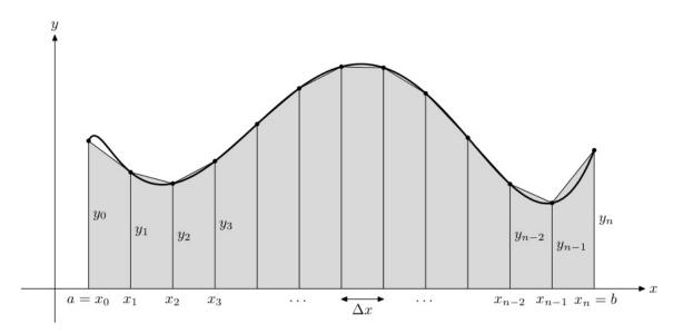
In the figure, the range [a, b] has been divided into *n* different trapezoids, each of which has the same base,  $\Delta x = (b - a)/n$ . Recall that a trapezoid with base *b* and sides *h*1 and *h*2 has area:
