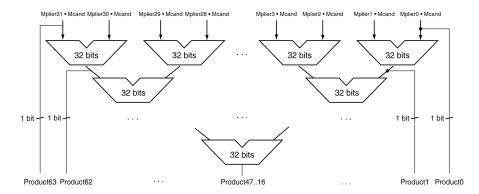
Determine the time required for a tree multiplier to multiply two 64-bit numbers if each step of the operation takes 4 ns. (The figure above describes a 32-bit multiplier.) Note that some of the hardware may be able to operate in parallel.
