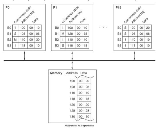
Each cache is direct-mapped, and each block contains two 32-bit words of memory—only the least significant byte of each word is shown. Addresses are written in hexadecimal. In this figure, the address tag shows the full address for simplicity. The coherence states are M (Modified—both exclusive and dirty), S (Shared), and I (Invalid). The system uses write-back caches and a write-invalidate protocol.
